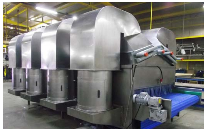
EVAPORATIVE COOLING TUNNEL
